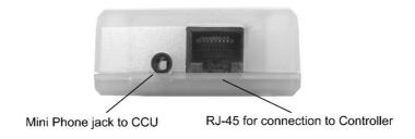
The RU-2 connects to the controller using the supplied short Ethernet style cable and to the CCU using the supplied 1/8" (3.5mm) 'pigtail' cable. Unless the CCU uses screw terminals you will need to attach the appropriate connector to the bare wires on the pigtail.
